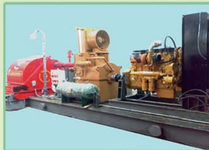
与卡特柴油机配套的偶合器机组 Coupling set matching with Caterpillar diesel engines
