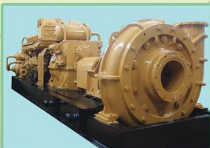
与济柴柴油机配套的泥沙泵偶合器机组 Sediment Pump Coupler Unit Matched with Jinchai Diesel Engine
