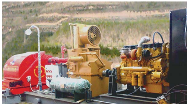
反车箱配卡特柴油机驱动泥浆泵实况 Scenario: Reverse-gear box with Caterpillar diesel engine to drive mud pump
