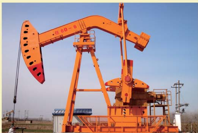
抽油机用液传动力装置在华北油田使用现场 The fluid transmitted power device for the pumping unit at the job site of North China Oil Field
