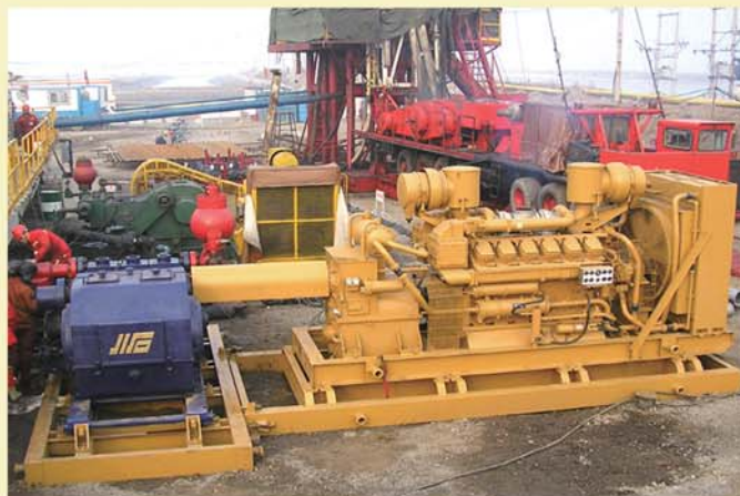
柴油机耦合器反车箱单机泵机组 Diesel engines coupling reverse-gear box single pump units
