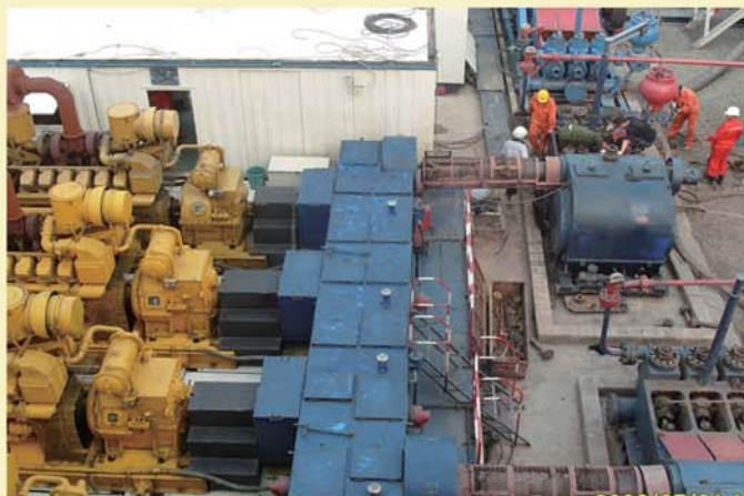
柴油机耦合器正车箱动力机组 Diesel engines coupling gear box power units
